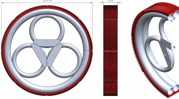
Fig. 4: Final Wheel Mode with 3-ring
