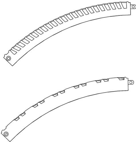
Fig. 9: Side view of the first tread design (top); and second tread design (bottom).
