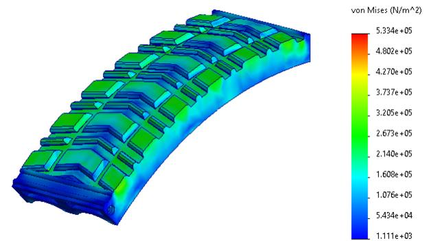
Fig. 7: Von Mises analysis of the second tread design.
