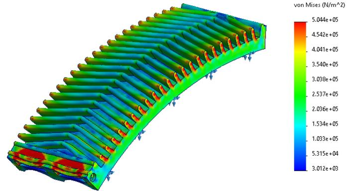
Fig. 6: Von Mises analysis of the first tread design.
