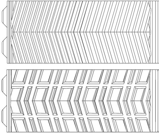
Fig. 8: Top view of the first tread design (top); and second tread design (bottom).
