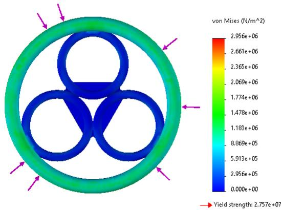
Fig. 5: Von Mises analysis of the wheel's aluminum ring.
